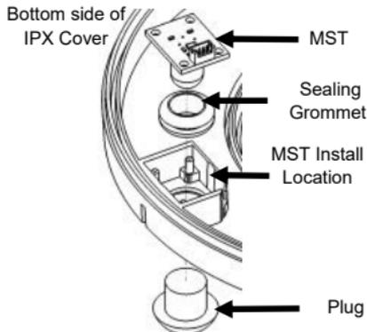
**MST1:** Remove the Plug already in the IPX cover. Replace with the Sealing Grommet.
