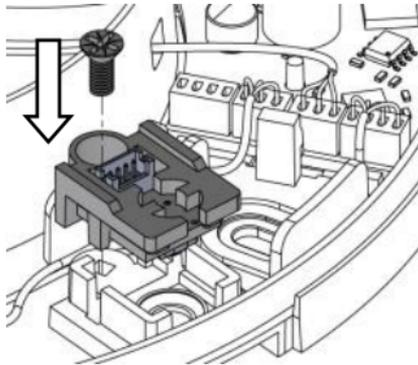
**HT2:** Place Humidity & Timer Module into the location shown above (the module will come with it's own holder) and screw into position.
