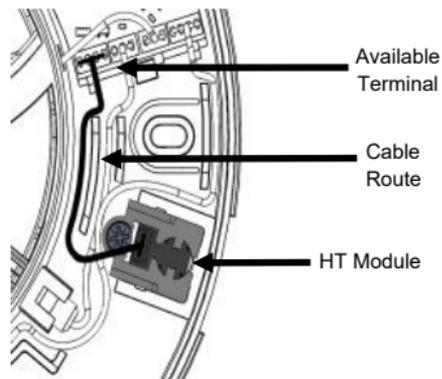
**HT3:** Attach the cable supplied into the Humidity & Timer Module and connect to the available terminal as labelled above.
