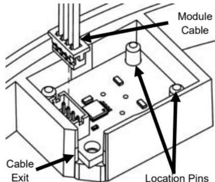
**MST2:** To position the MST module, ensure the location pins line up and press firmly into Sealing Grommet. Plug the cable provided into the MST module once secured in IPX cover.
