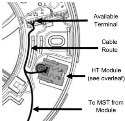
**MST3:** Connect this cable from MST into available terminal on the main body.
