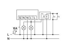
A maximum of 10 devices can be connected in parallel.
