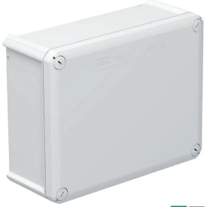
Junction box for the connection of cables and lines indoors and in protected outdoor areas. Rectangular design without entries. Suitable for wall and ceiling mounting, on mounting panels and threads in the floor. With the option to fasten inside and to mount via the corner domes. Cover with quick lock, sealable. Made from halogen-free materials.
